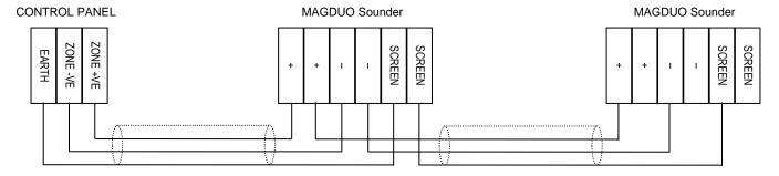
MAGDUO Sounders can be mixed on the same zone as other types of MAGDUO. The above diagram shows how to make the zone positive, zone negative and screen connections between the control panel and MAGDUO Sounders. Refer to the instruction leaflets supplied with other MAGDUO devices for their equivalent wiring/terminal labelling details.
