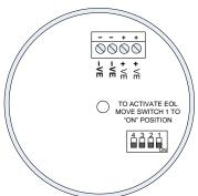
Once all testing has been carried out on the cabling and **continuity & insulation** has been proven, the Sounder front may be fitted. The Sounder front is fitted by locating the rubber seal in the groove on the back box and then pushing the front unit gently home. The four fixing screws may then be tightened as required.
